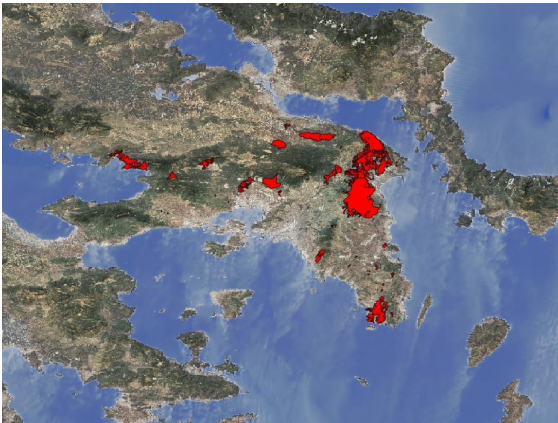
Burn Scar Mapping (BSM) data: derived from Landsat TM Imagery. Burned areas are represented with red polygons. Background image: Landsat Mosaic
